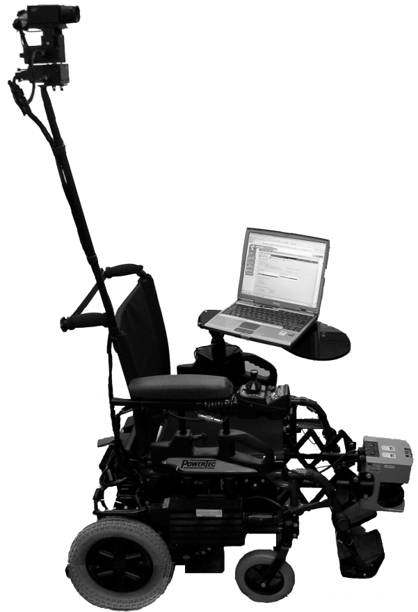
Figure 1. The SENA robotic wheelchair. While designing SENA , we have paid special attention to the positioning of the onboard sensors and devices in order to keep as free as possible the user space while preserving their functionality.
