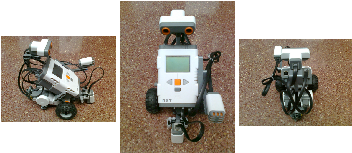
Figure 1. NXT physical configuration used in all the courses.
